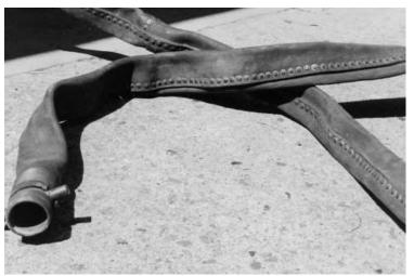
Picture of one of the original leather hoses showing the brass studs used to seal the joint. The hose was very heavy even when empty and dry
