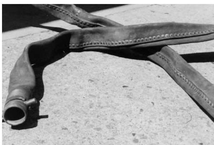
Picture of one of the original leather hoses showing the brass studs used to seal the joint.
